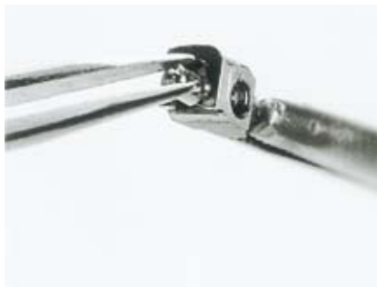
17 Remove the lock bolt and compression spring.
