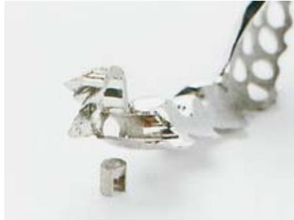
**25** Sandblast the threaded cap and the threaded cap recess in the CrCo framework with 250 µm corundum at approx. 5 bar pressure. Remove the block out wax with a steam cleaner.
